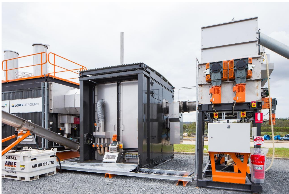
Demonstration plant located at Loganholme wastewater treatment plant, showing the hearth unit where biosolids are thermally treated. Image courtesy of Pyrocal
